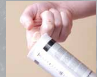
4 & 5: Pull off the cap on the other side of the cartridge
