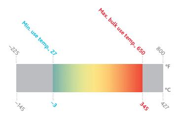
Eastman Therminol<sup>®</sup> 66 heat transfer fluid offers outstanding high-temperature performance to 345°C (650°F), including excellent thermal stability and low vapor pressure. These properties result in reliable, consistent performance of heat transfer systems over long periods of time. Therminol 66 performance is proven through many years of industrial experience under a wide range of operating conditions. No heat transfer fluid material in the world has had more success than Therminol 66.
